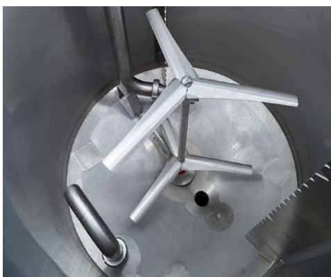
Mixing container designed for heavy viscous gravies/mixtures. The Ytron and the Venturi system in combination with the Heavy Duty mixing agitators ensure a fast processing of a gravy free from lumps. Anti-vortex breakers are standard in all scanGravy mixing tanks. Direct steam injection for temperature control can be added as well.
