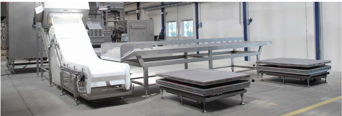
Belt Conveyor with unpacking station with 2 (two) lifting tables for ergonomics, left side.
