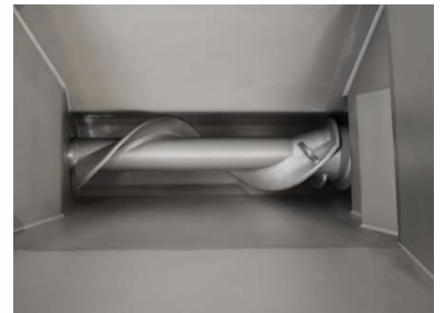
Infeed hopper shown from top view. Please note the grinding worm/auger with the sharp knife edge, designed to grab and feed both frozen blocks and fresh meat raw materials.
