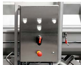
Standard screw conveyor electrical/operator panel.
