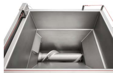
Infeed hopper shown from top view.
