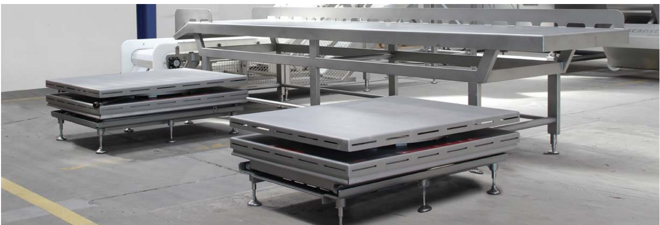
Belt Conveyor with Unpacking station with 2 (two) lifting tables for ergonomics, right side.
