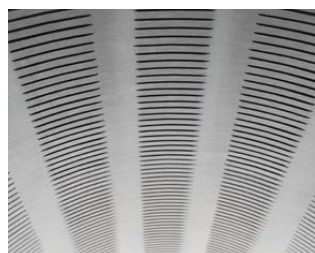
Slit filter seen from inside.
