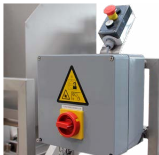
Operator/control panel with emergency stop.
