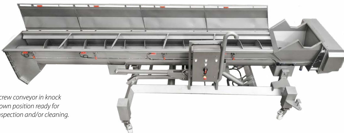
Example of infeed section for grinder.
