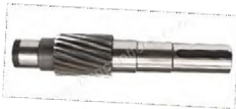
Pinion shaft for C.400/B.400 gear box, part number 5000037647 / 37647
