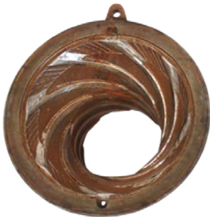
Lining for Simo® grinder before refurbishment
