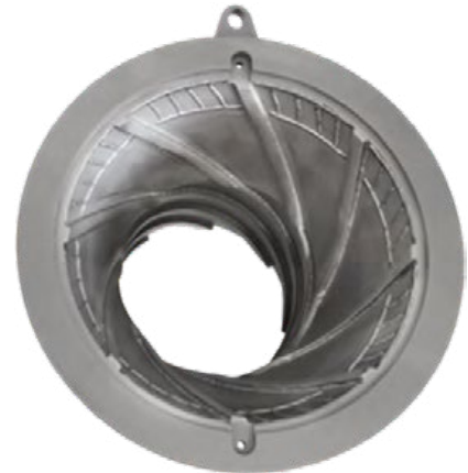
Lining for Simo® grinder refurbished
