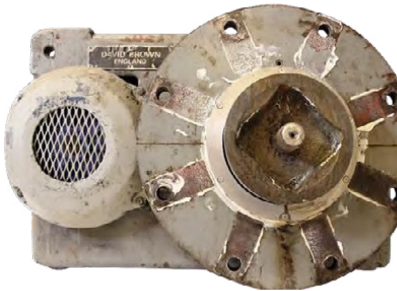
David Brown gear box before refurbishment
