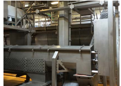
scansteel foodtech Whole Pallet Crusher, WPC 2000-Single, shown in application where existing footprint is sparse and where the pre-broken frozen blocks must be elevated to approx. 5000 mm.
