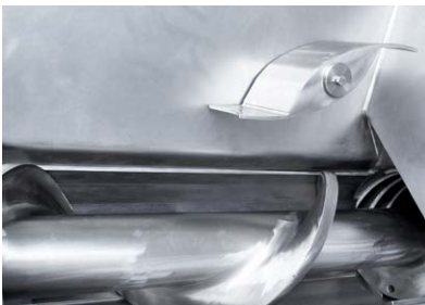
Cheese feed guide shown right mounted. Electro polished feeding worm/auger, also shown.
