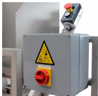
Operator/control panel with emergency stop.0+
