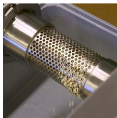
Cheese extrusion filter comes with varied filter sizes, typically Ø2.8, Ø5 and Ø14 mm.
