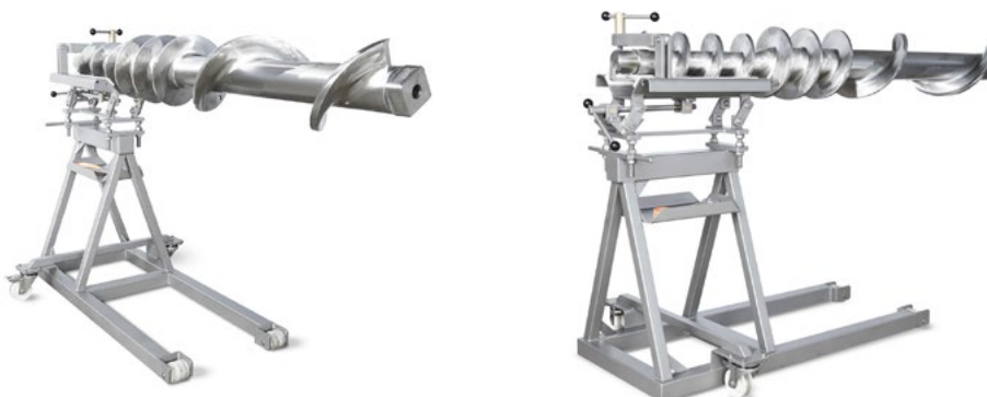
Removal of breaker worm for CombiGrind CG 225, CG 300, CG 300 Heavy Duty.
