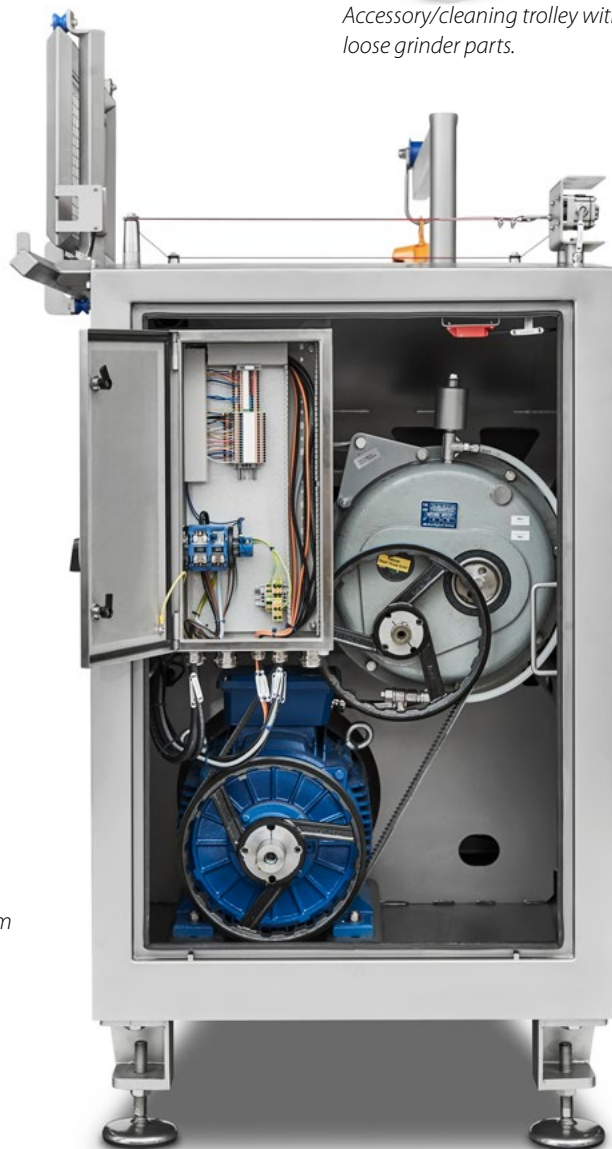
A prime example of scansteel foodtech's hygienic design is given by the hygienic zone positioned between the worm/auger and the gear box. Hygienic zone shown in running position (closed) and in cleaning/inspection position. When opened the grinder cannot be started until the guard is positioned in closed position. = When opened, the grinder cannot be started until the guard has been positioned in closed position.
