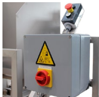
Operator / control panel with emergency stop.
