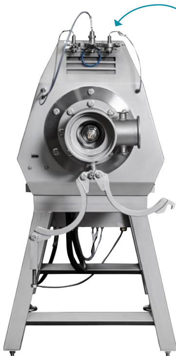
scanEmul 175 shown disassembled, ready for cleaning, front view.
