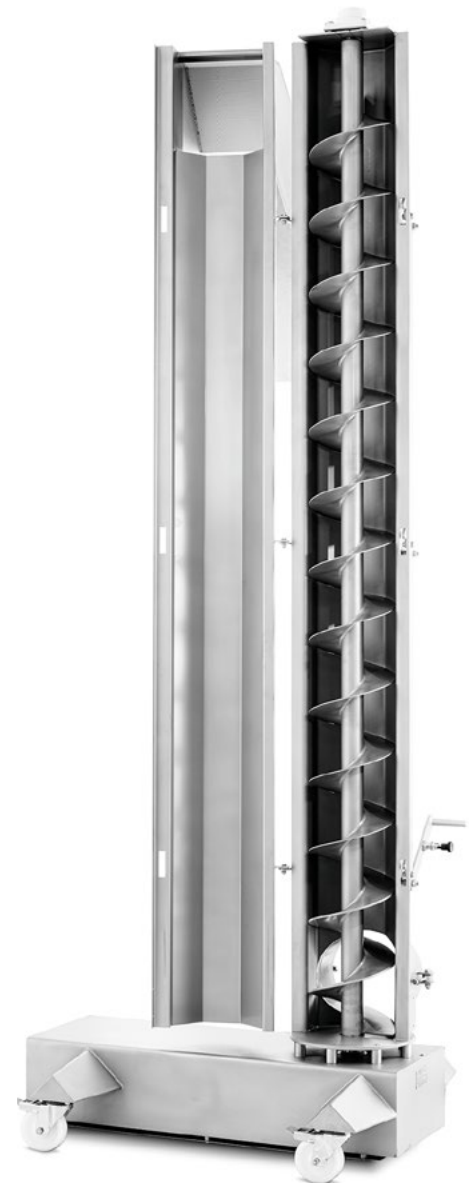
scansteel foodtech standard scanGiraff, showing vertical screw.
