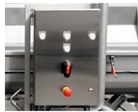
Standard screw conveyor electrical/operator panel.
