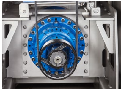
Planetary gear box assembly. Between gear box and crusher claw, a Heavy Duty safety clutch prevents damage to the gear box, example only, in case a large foreign (metal) object by mistake is thrown into the Whole Pallet Crusher.
