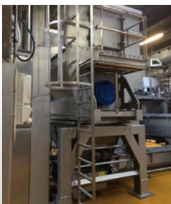
Final installation of Whole Pallet Crusher, WPC 2000-Single, at customer site, shown with platform with ladder.
