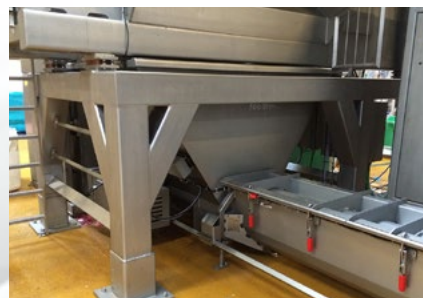
Horizontal screw shown with closed lid.
