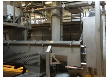
scansteel foodtech Whole Pallet Crusher, WPC 2000-Single, shown in application where existing footprint is sparse and where the pre-broken frozen blocks need to be elevated to approx. 5000 mm.
