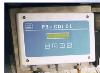
Detergent dosing device with concentration control and LCD display.
