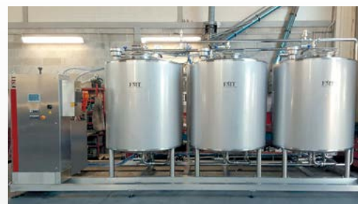
CIP cleaning system
